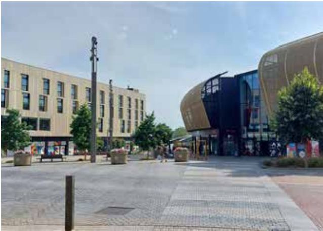
The design of the square subtly incorporates the vehicular route without compromising the quality of the public realm with a carriageway level with surrounding paving, using material changes and subtle detailing, creating a pedestrian priority environment. (Elwick Road, Ashford.)
